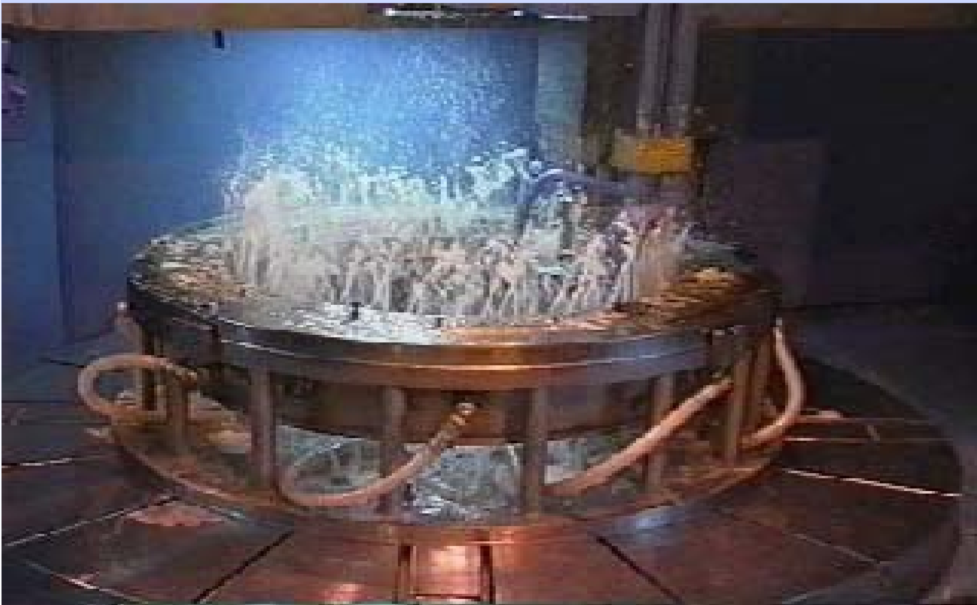
Grinding the nose of the largest commercial jet engine 800 l/min coolant through the table to the fixture to ensure dust free
