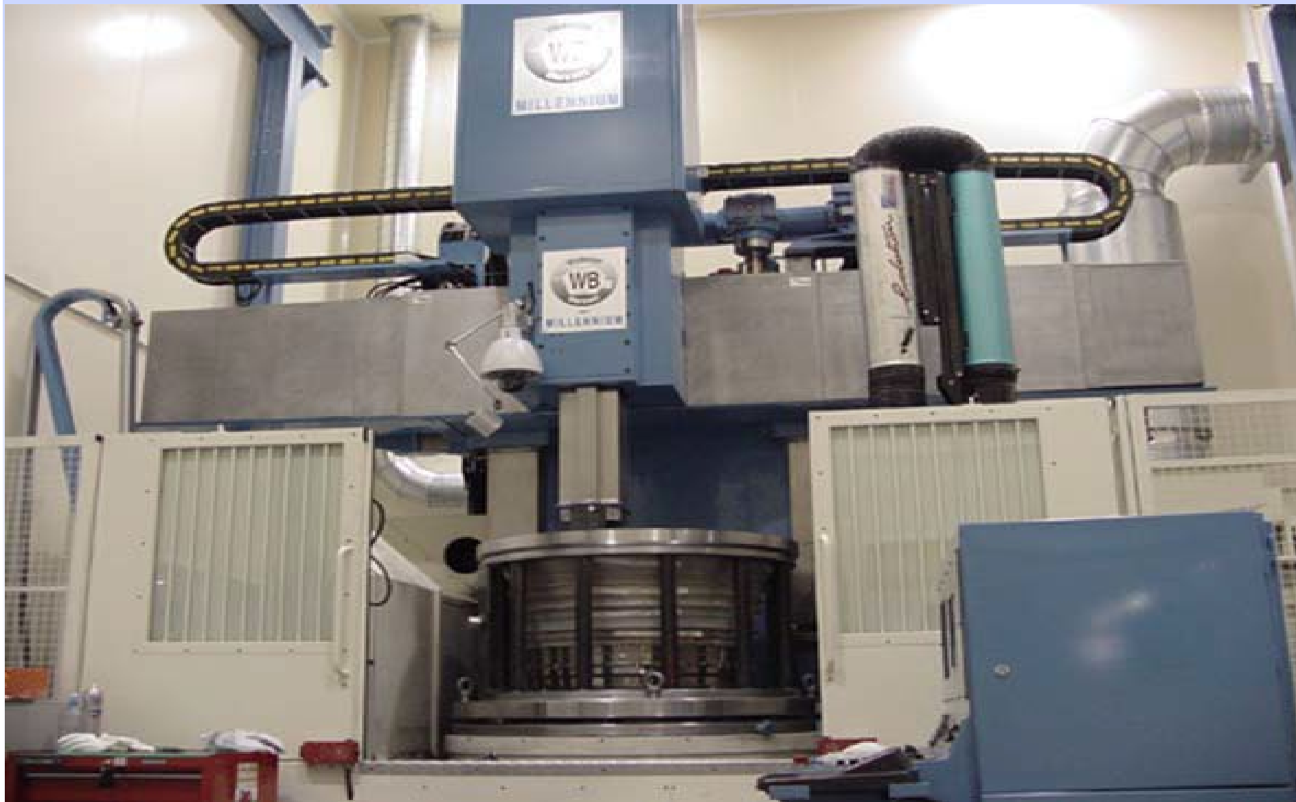
TURNING AERO ENGINE CASINGS (INTERNAL) – ACCURACY 7 \mu
