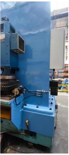
Good day. Happy with the checkover of the motor, gearbox and gear changer – so re assembled it. The four controls on the left of the first picture are flow control valves for the excellent and powerful lubricating system for the chain drive and sprocket bearing assemblies, the Andantex gearbox and the huge Timken cross roller table spindle bearing
