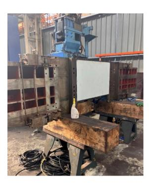
At the back of the crossrail the cable chains, pipes, hoses, cables, connector boxes an wiring have been removed and will be reassembled in a 2020's format.
