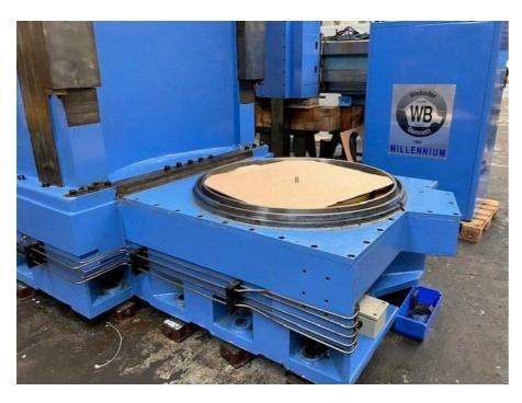
Inside the casting and underneath the temporary protective covers is another component that epitomizes the Millennium quality – the wonderful **TIMKEN** crossed roller table bearing. More than 50 years ago Timken developed these bearings for Webster & Bennett heavy duty double column machines with huge 3,600mm diameter tables. With a perfect performance record it was no wonder we specified them when we were designing the Millennium
