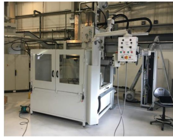
2016 – another with pendant controlled power swivel to the ram
