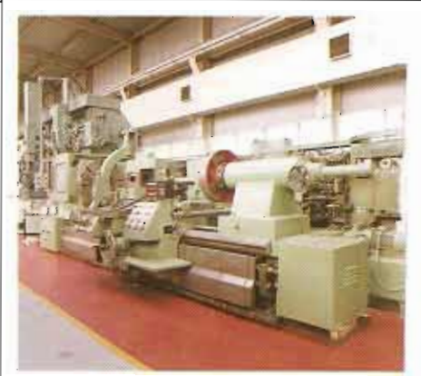
CRAWFORD SWIFT LATHE, 1982. 120" BETWEEN CHUCKS/CENTRES
