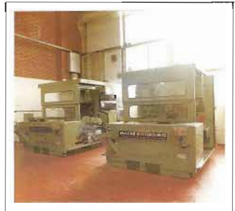
MAZAK H10 TWIN PALLET, 1982, HORIZONTAL WITH FANUC 6M & 6MB WITH DNC. CAPACITY 560mm x 400mm x 400mm. 24 TOOL ATC 10 HP. 72 POSITION INDEXING PALLET
