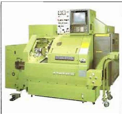
HITACHI-SEIKI HI TECH 20 D, 1986, WITH FANUC 10TF. CAPACITY TURRET TRAVEL 340mm. CROSS 170mm. 12 POSITION TURRET. BAR CAP 45mm
