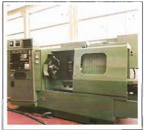
TAKISAWA TX2 WITH FANUC 6TB, 1982. 490mm x 600mm
