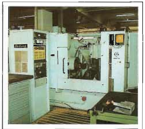
FORTUNA CNC CHUCKING GRINDER, 1985. FANTASTIC MACHINE - ANGLE HEAD 900mm DIA. WHEEL. 50 kW MOTOR. MARPOS MEASURING. EXTREMELY FULLY EQUIPPED. SEND FOR FULL INFORMATION OF THIS HALF PRICE OPPORTUNITY.
