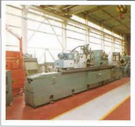
CINCINNATI 14' x 80", 1974 GRINDING MACHINE WITH ACCRASIZE
