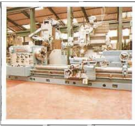
TUDA JUMBO OIL COUNTRY - UNUSED - LATHE. 700mm SWING x 3 METRES
