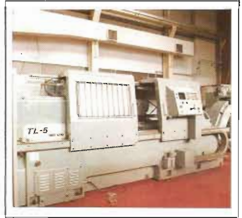
MORI SEIKI TL5A YASNAC 20006, 1982. CHUCK DIA. 300mm. MAX. TURNING LENGTH 1950mm. MAX. WORKPIECE DIA. 280mm. 8 POSITION TURRET. PROGRAMMABLE TAILSTOCK, 18.5kW
