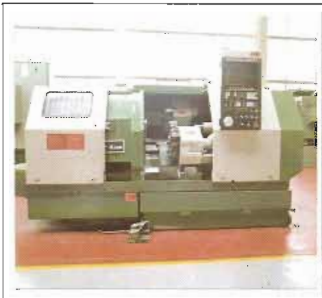
YAMAZAKI Q-SL 20 – 4 AXIS WITH CAM T4 CNC. MAX. TURNING LENGTH 500mm. MAX WORKPIECE DIA. 220mm. CHUCK DIA. 200mm. 2 x 8 POSITION TURRETS 25 HP
