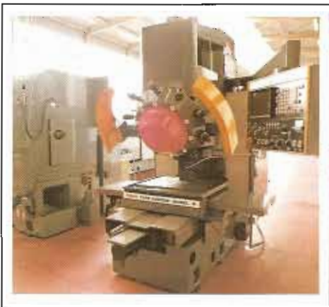
FANUC TYPE D - 10 SPINDLE TURRET MACHINE WITH FANUC 6MB. 500mm x 380mm x 400mm. DRILLING 25mm. TAPPING DOWN. END MILLING 40cm 3 /min (MILD STEEL)
