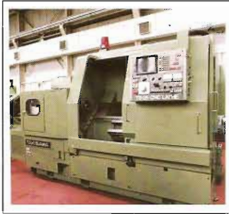
TAKISAWA TS25 WITH FANUC 6TB. 33 KVA. 4000 rpm
