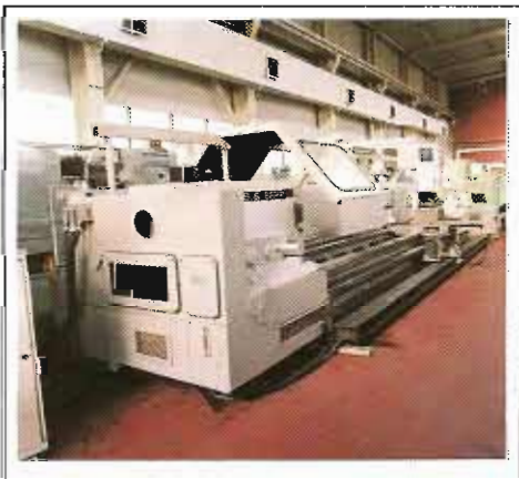
BINNS & BERRY TRIDENT 80-850 WITH ALLEN BRADLEY 8400 CNC. 850 x 5500mm, 40 hp, 1984
