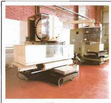
AMADA BM114 VERTICAL, 1982, WITH FANUC 6MB. 24 TOOL ATC. TABLE SIZE 1098mm x 400mm
