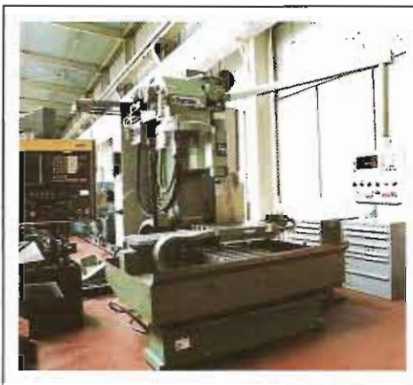
CHIRON FZ25 MACHINING CENTRE WITH SINUMERIK 6M, 1981
