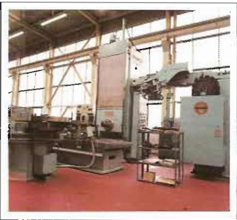
SUNDSTRAND SERIES 80, 1977. MODEL H45-SC. HORIZONTAL WITH DEC PP11 MINI COMPUTER. CAPACITY X - 48" Y - 36" Z - 80". 32" DIA. CONTOURING TABLE. 40 TOOL ATC. AUTOMATIC PALLET CHANGE
