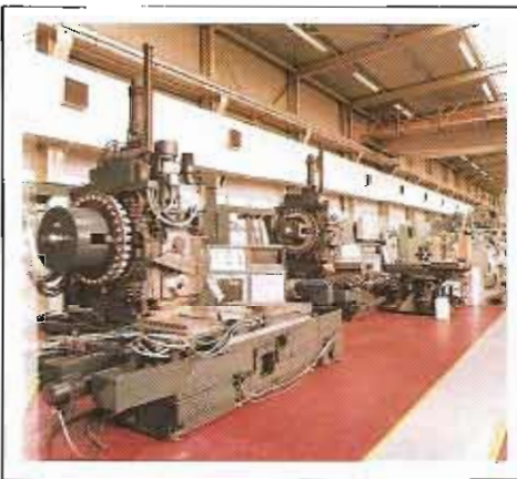
CINCINNATI HC20/1250, 1978, 4 AXIS HORIZONTAL, CINCINNATI "BIG BLUE CNC". TWIN 28" PALLETS ON ONE MACHINE. BUILT-IN 30" ROTARY ON OTHER MACHINE. 30 POSITION ATC. IN PROCESS OF RECONDITIONING
