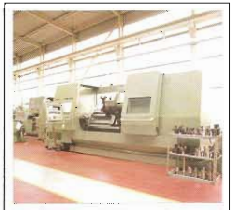
GILDEMEISTER MD10S WITH ELTROPLOT M, 1982. 2 AXIS. LONG TRAVEL 2058mm. MAX. TURNING DIA. 440mm. SWING OVER BED 655. CHUCK DIA. 400mm. PROGRAMMABLE STEADIES
