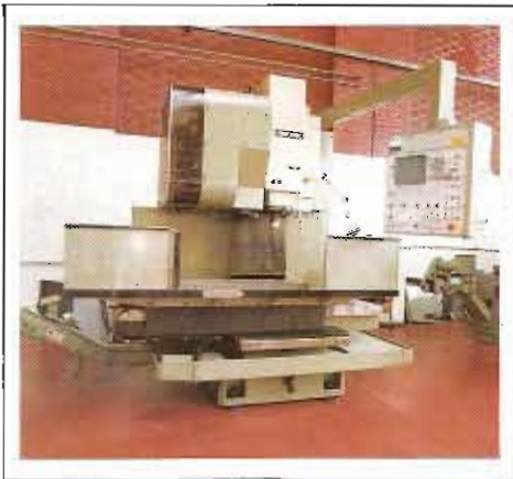
MORI SEIKI MV 35-40 VERTICAL, 1984, WITH FANUC 6MB. 20 TOOL ATC 762mm x 350mm x 450mm, 5.5kW
