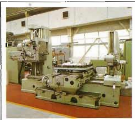
TOS WB63 HORIZONTAL BORER, 1978. OPTICS
