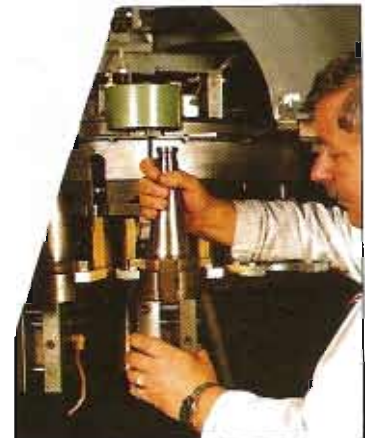
Loading tooling into automatic toolchanger
