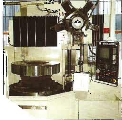
1st operation on Weld Neck Flange – 48 inch 'TXE' machine
