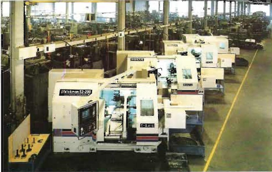
A versatile range of 2, 4, 5 & 7 axis turning centres with the ability to perform simultaneous operations and finish components on a single machine, with power tooling and 'C' axis control. Machines can be supplied with gantry and other types of loading to suit customers requirements.
