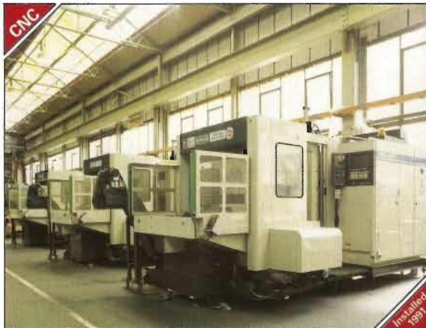
Shibaura Toshiba 'BMC 50E' CNC Twin Pallet Horizontal Machining Centre with Tosnuc '800 M' CNC Control
