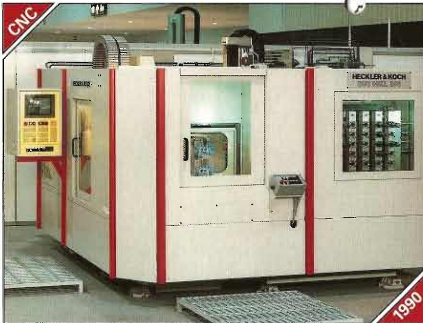
Heckler & Koch 'Duo Mill 200' CNC Twin Spindle Horizontal Machining Centre with Heckler & Koch 'CNC 785-M' Control
