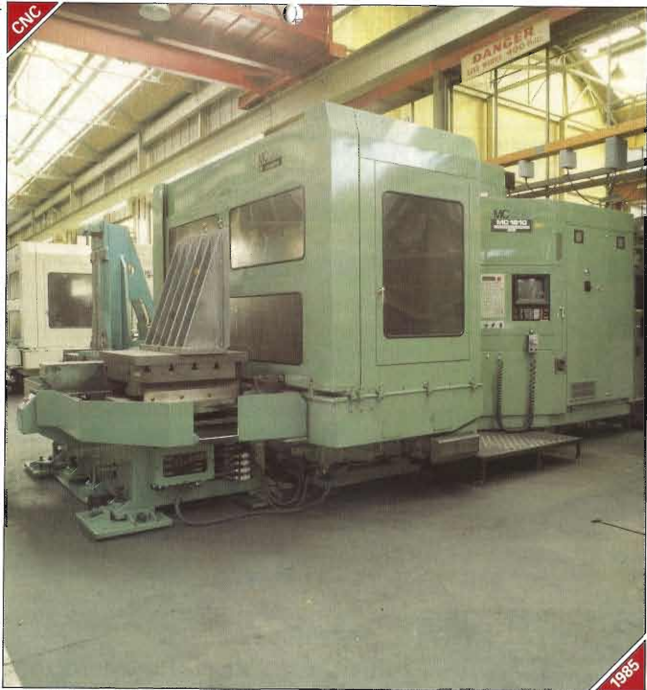
Makino 'MC1210' Twin Pallet Horizontal Machining Centre, with 800 x 800mm Pallet size and Fanuc '6MB' CNC Control
