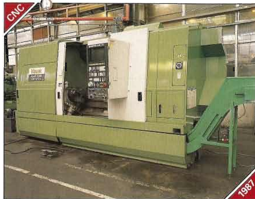
Mazak '40N-ATC' Slant Turn Mill Centre with Mazatrol 'CAM T3' CNC Control
