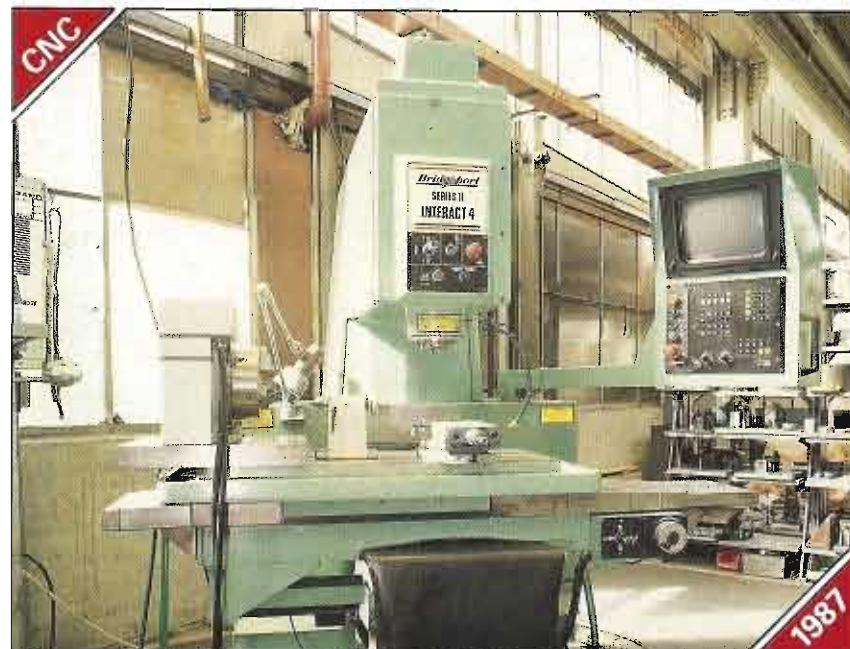
Bridgeport 'Series II Interact 4' CNC Vertical Milling Machine with Heidenhain 'TNC 151' CNC Control
