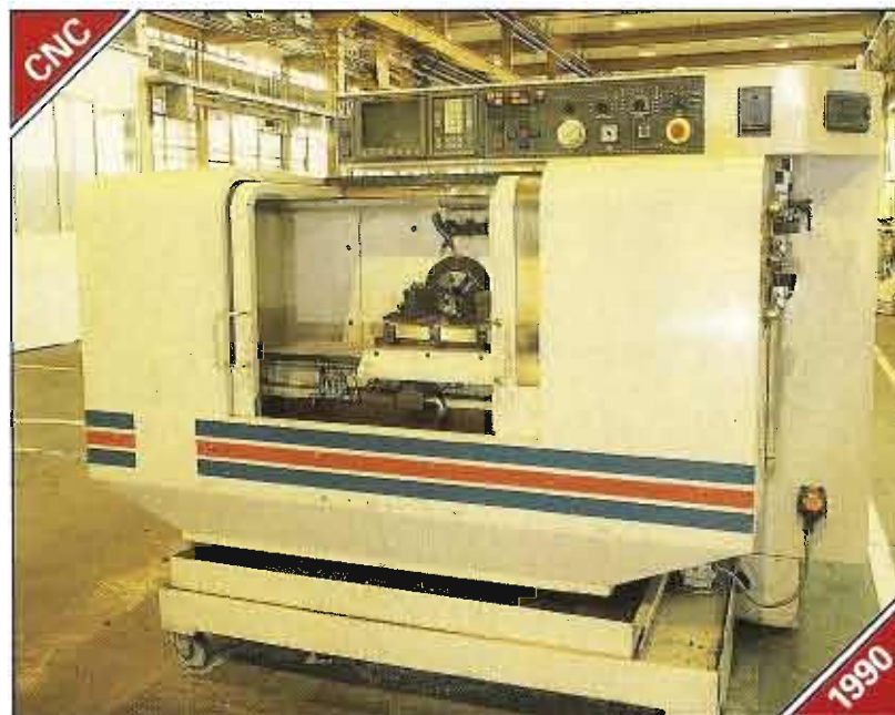
Wickman 'KIS 26/130' CNC Bar and Chucking Lathe with Fanuc 'OT' CNC Control
