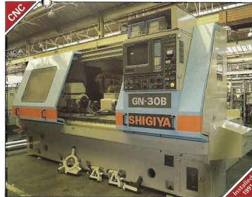
Shigiya 'GN 30B' CNC Angle-Head Cylindrical Grinder with Fanuc 'OOGC' CNC Control
