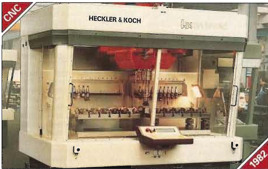
Heckler & Koch 'BA20' Twin Pallet Vertical Machining Centre with Heckler & Koch '781' CNC Control
