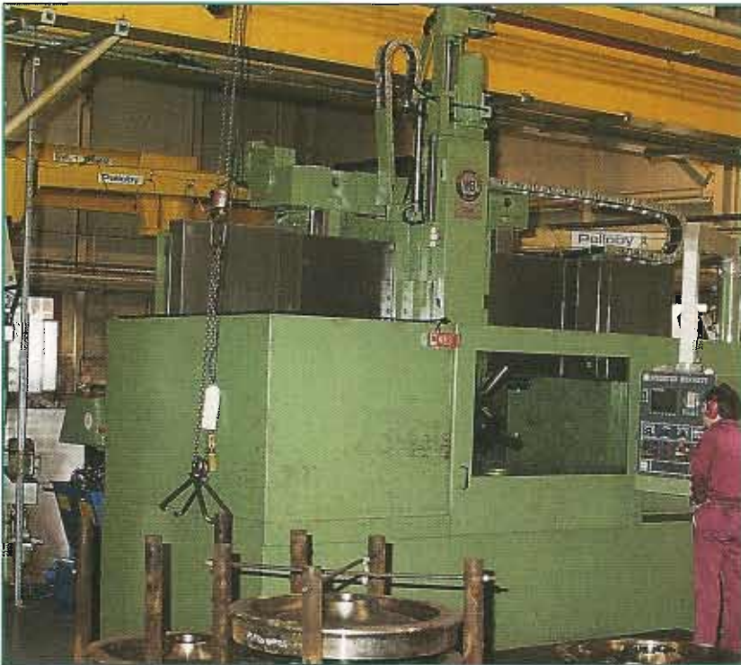
Webster & Bennett Titan 1200 Turning Railway Wheels in London
