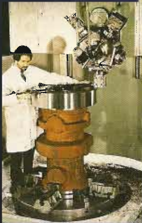
Oilfield Pipeline Valve Body
