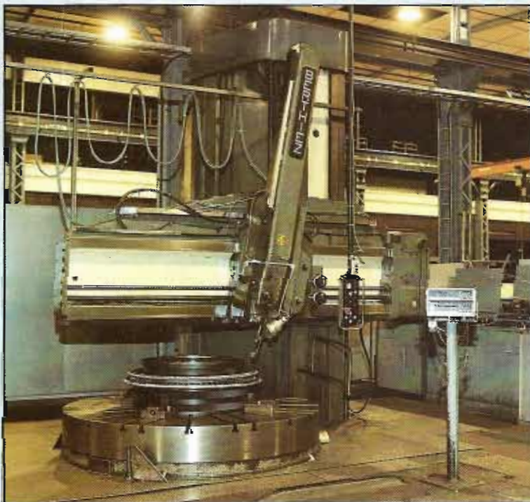
BERTHIEZ BM 225 OPENSIDE VERTICAL BORER. Retractable Table 2250 mm diameter. SWING 4500 mm. Maximum height 200 mm. 1-100 rpm. PENDANT. NEW 1959. EXCELLENT. Fitted DIGITAL READOUT.
