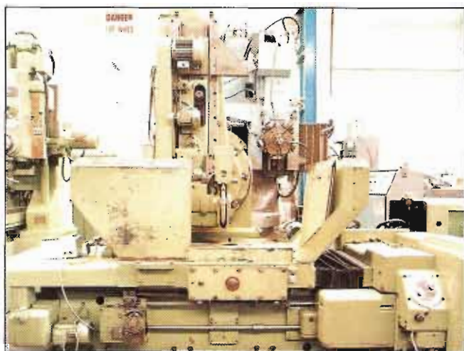
NILES ZSTZ 800. New 1965. 800 mm diameter. 2- 14 Modul. 45° helical. 2000 kg table load. Well equipped. £14,500.
