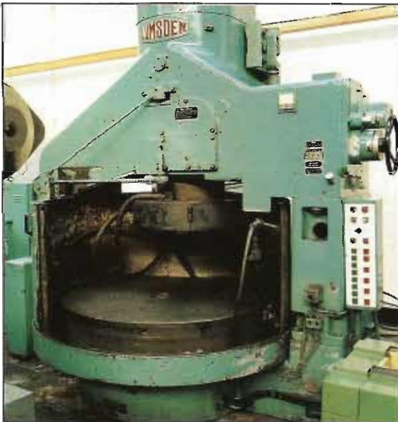
LUMSDEN 93ML VERTICAL SURFACE. 60" magnetic chuck. 60 h.p. 1975 — £22,000.
