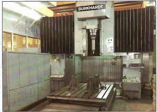
BURKHARDT JIG BORER. 2500 mm x 1850 mm. 2500 mm between columns. Accepts 17 tons on table. 1969 — MAGNIFICENT — £35,000.
