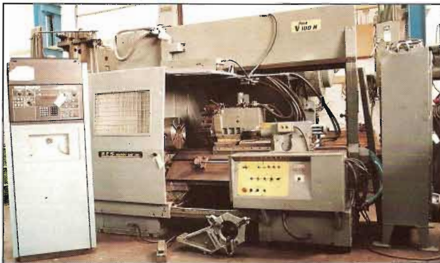
H.E.S. V100N CNC LATHE 510 mm swing x 1250 mm centres. 26KW motor. G.E. 1050 CNC. NEW 1978. EXCELLENT. £26,000.
