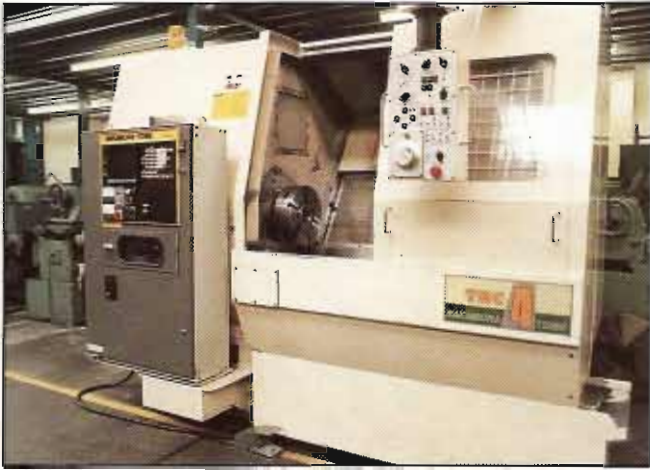
NAKAMURA TMC4 CNC LATHE. 400 mm swing. 300 mm chuck. PROGRAMMABLE TAILSTOCK. 12 position Tool Turret. FANUC 6TB with C.R.T. Display. NEW 1981.
