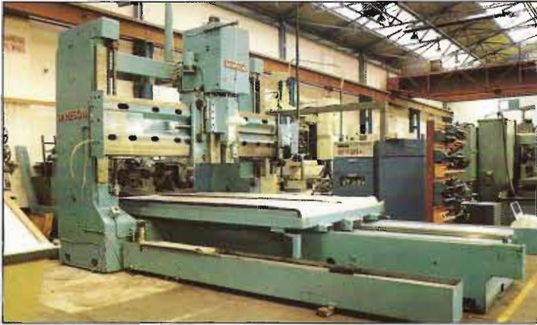
JAMESON F487 MILLING and BORING MACHINE. Table 126" x 66". 31-1808 rpm. 1979 — fitted DATASAAB MTC 9 control. Absolutely Superb. £35,000.
