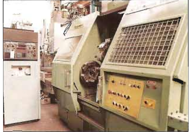
H.E.S. TRANSUM CNC LATHE. 500 mm swing. 325 mm length. G.E. 1050 C.N.C. NEW 1980. £26,000.
