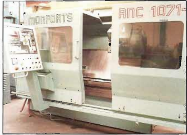
MONFORTS RNC 1071 E CNC LATHE. At present set up for collet loading. Can be set up also for chucking. 12 position tool turret. 22KW d.c. drive. G.E.1050 CNC. NEW 1980. PERFECT. £32,500.
