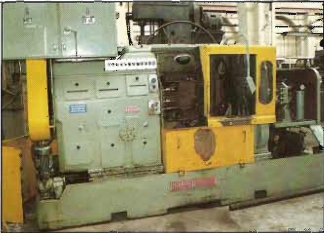
HERBERT — BSA GRIDLEY 8 spindle 6 inch chucks. Double indexing. New 1971 £12,750
