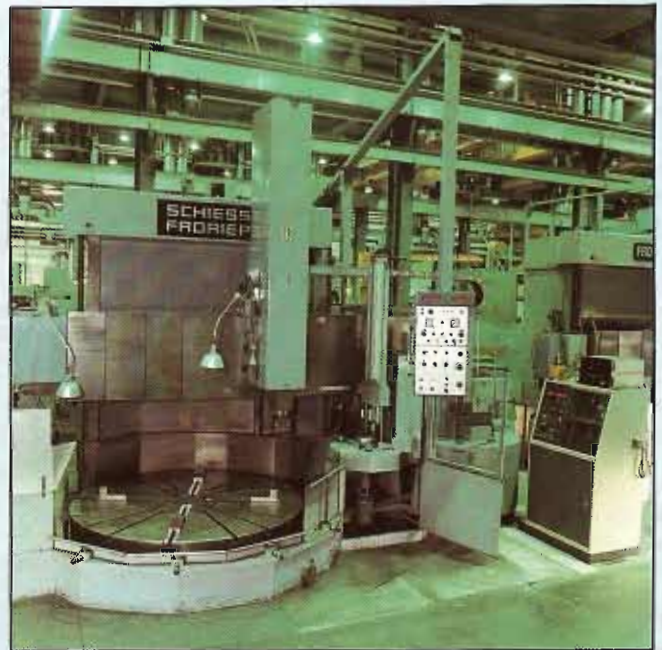
SCHIESS FRORIEP DS 20 N.C. VERTICAL BORER with AUTOMATIC TOOLCHANGER — 32 station. Table 2250 mm diameter. Swing 2500 mm. Max height 1600 mm. Maximum table loading 12.5 tons. 2-160 rpm. BOSCH 800 N.C. Continuous Path. NEW 1973. EXCELLENT + similar 1971 machine also available.
