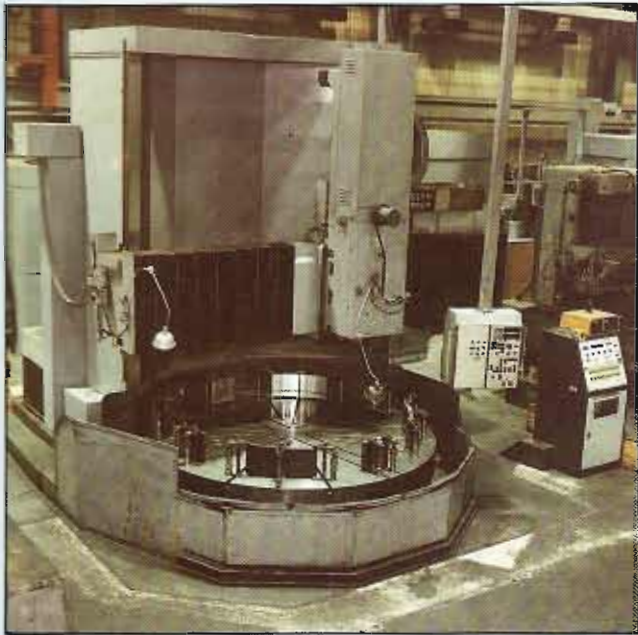
SCHIESS FRORIEP 32 DE 300 N.C. VERTICAL BORER. Table 3000 mm diameter. Swing 3200 mm. Max height 2500 mm. Maximum table loading 20 tons 1-100 rpm. ASEA NUCON 312 Continuous Path Numerical Control. NEW 1974. EXCELLENT. At a fraction of replacement cost.
