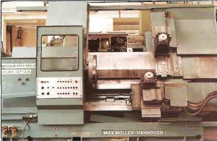
GILDEMEISTER MDR32-4A N.C. LATHE. Swing 830 mm. 1280 mm turning length. 128 mm spindle. 650 mm chuck. Swarf conveyor. 50 h.p. NEW 1973. SINUMERIK N.C. £14,000.
