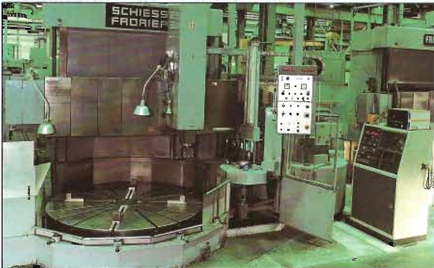
SCHIESS FRORIEP DS 20 N.C. VERTICAL BORER with AUTOMATIC TOOLCHANGER — 32 station.
