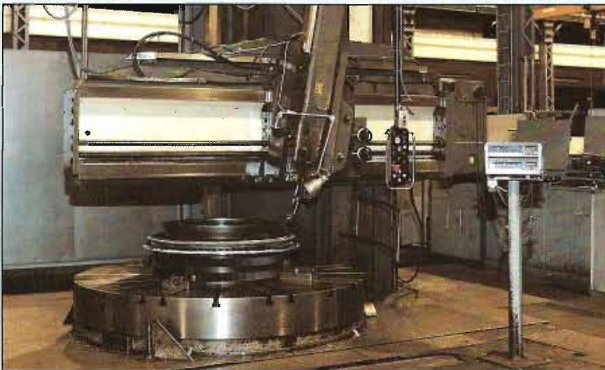
BERTHIEZ BM 225 OPENSIDE VERTICAL BORER. Retractable Table 2250 mm diameter. SWING 4500 mm. Maximum height 200 mm. 1-100 rpm. PENDANT.
