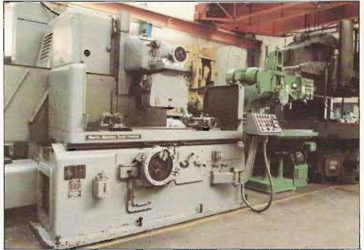
1972 MATRIX-THOMPSON CT11 Truforming & Creep feed Grinder Capacity 36" x 12" (magnetic chuck) x 16" under wheel. 20 hp. wheel head.
